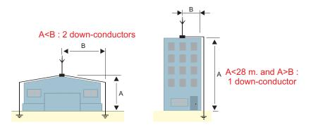
The path has to be the most rectilinear possible with the shortest distance, avoiding curves. The covering radius should not be less than 20 cm. The down-conductor should avoid crossing or the proximity of electrical or telecommunication networks.
