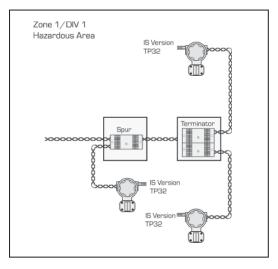
Install TP32-X-NDI (where X =thread type) on **every** instrument critical to the operation of the process.
