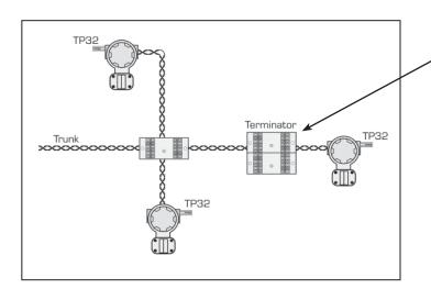
Junction block and terminator are required at the far end of a Fieldbus trunk.
