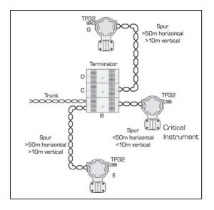
Install a TP32 on every instrument critical to the operation of the process system.
