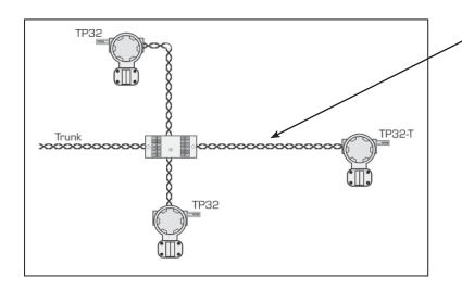
Use of TP32-T eliminates the need for an extra junction block and terminator.
