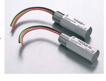
exposed to damaging transients between the lines and ground. Any surge current appearing as a series-mode or common-mode transient is converted into a common-mode voltage whereupon the transmitter electronics are temporarily raised to some higher voltage level before 'floating' down automatically (and without damage) to resume normal operation.
