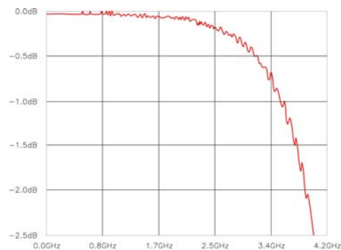
Figure 2 Typical attenuation plot for N-type CA devices
