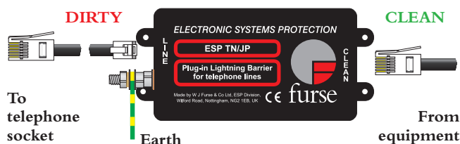
Plug-in series connection for ESP TN/JP (above) and ESP TN/RJ11-2/6, 4/6 & 6/6 (below) and ESP ISDN/RJ45-4/8 & 8/8 (bottom).
