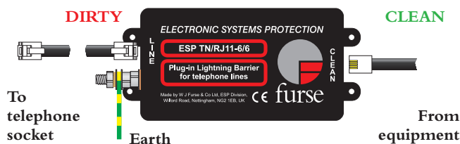
Plug-in series connection for ESP TN/JP (above) and ESP TN/RJ11-2/6, 4/6 & 6/6 (below) and ESP ISDN/RJ45-4/8 & 8/8 (bottom).
