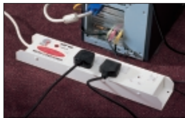
ESP MC installed at floor level protecting a PC and monitor.
