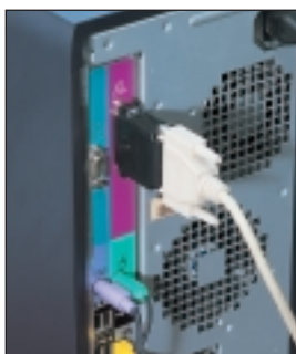
ESP LA-5/25 installed on the parallel port of a PC, protecting the printer connection.
